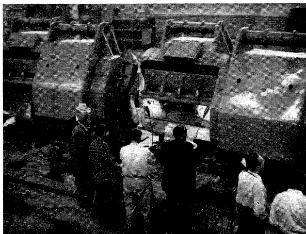
After the Kiev Conference, some CERN scientists visited Prof. Alkhanov's Institute in Moscow where a 7 GeV accelerator is being installed. This photo shows the magnet units being aligned. Note their special shape - an open C. (C. J. Bakker photo.)
